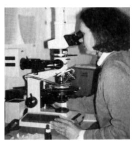
A complete paint investigation often needs to be conducted during Restoration. Paint samples are carefully collected onsite. In the laboratory, an ultra violet light is used to identify pigment and binding media. Paint samples are then photographed. Physical evidence documented through laboratory research provides a sound basis for an accurate restoration of painted finishes, such as the complex stencilling pictured here. Photo left: Courtesy, Alexis Elza; Photo right: Courtesy, Andrea Gilmore.
